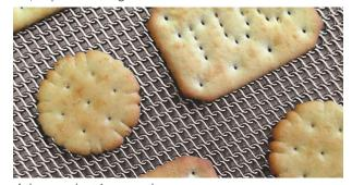
breakage and packing is facilitated, since the bottom side of the product is smooth.
